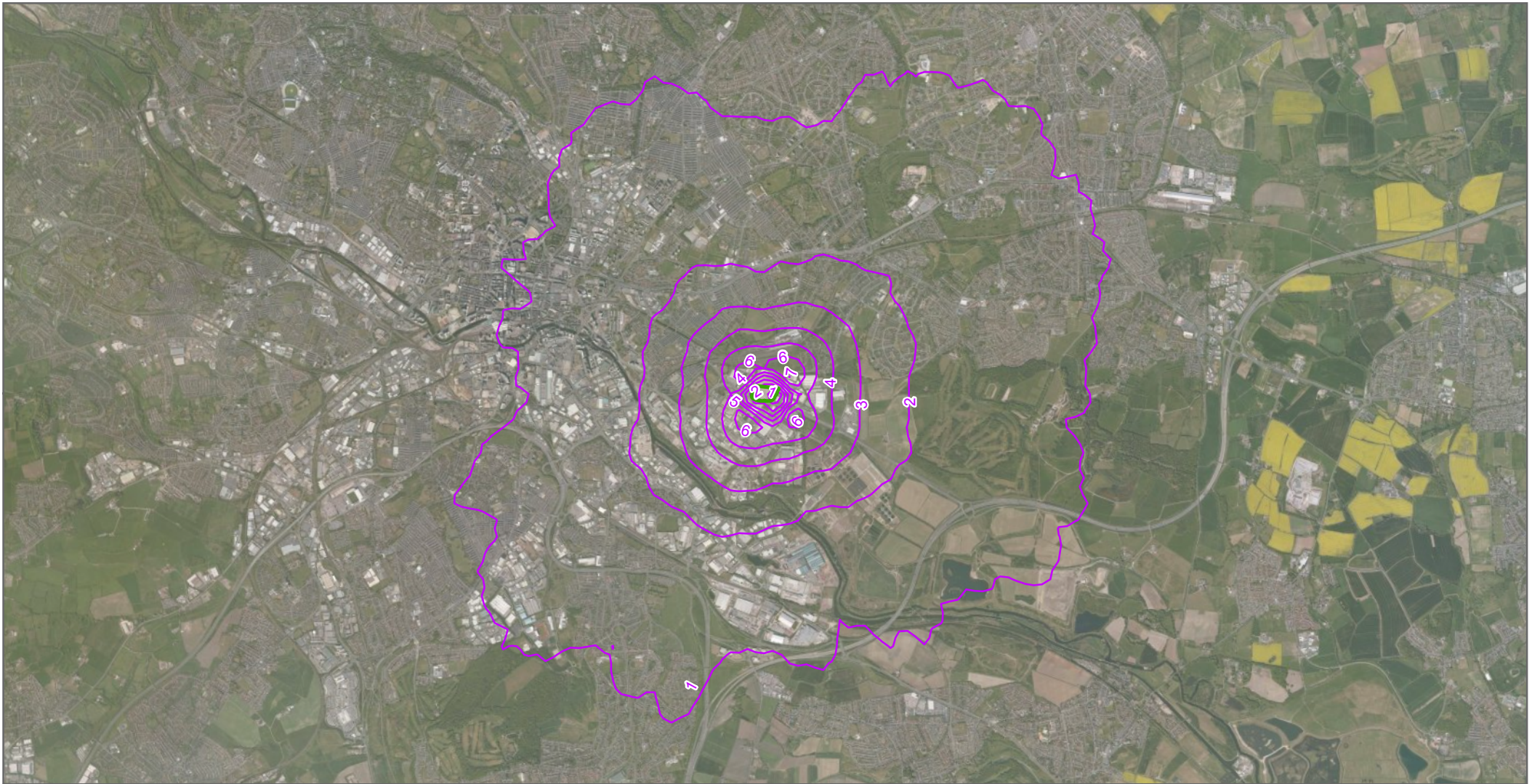
Figure D3.4 Predicted 99.8th Percentile of Hourly Mean NO 2 Concentrations ( \mu\text{g}/\text{m}^3 )
